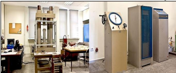
In this laboratory physical and mechanical properties of rock samples, taken from the surrounding rocks of underground structures (galleries, tunnels, underground openings) and natural building stones like marble, travertine, are determined.
