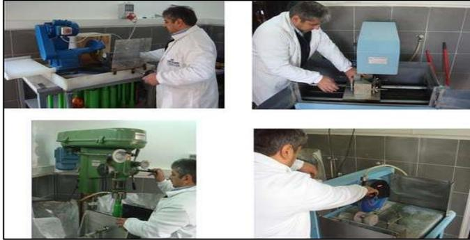
This laboratory is used to prepare rock specimens for mine machinery and mechanization laboratory in order to determine the cuttability and wearability of rocks.
